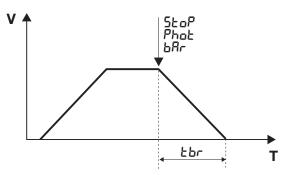
The intervention of the safety input causes an immediate slowing of the gate, the time in which the gate switches from standard speed to a complete stop is adjustable through the TBR value and must respect the values indicated in Table 1. **IMPORTANT:**
