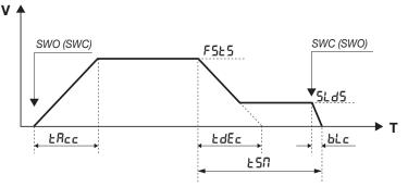
The V axis is the gate/door speed, T axis is the time required by the door/gate to move from a limit switch to the other. The parameters govern both the opening and the closing phases.
