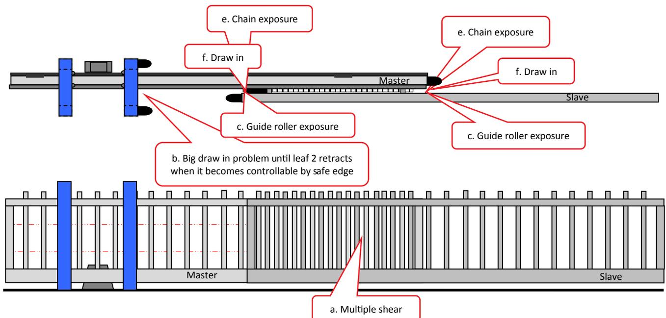
**C** Guide roller exposure can lead to finger traps as with conventional sliding gates but is exemplified because the guide channel and rollers between master and slave leaf are more exposed and move with the leaves. The solution could be local guard or enclosure of channel, see drawing below.
